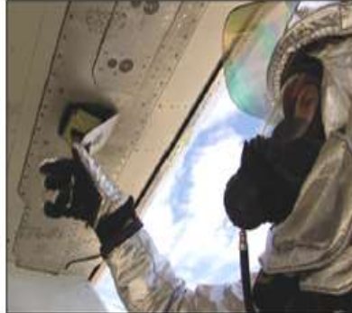
Step 2: Gain access to fuel valve for that line.
